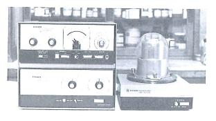
Quantitative differential thermal analysis used in "finger-printing" materials having characteristic transition and decomposition temperatures.
